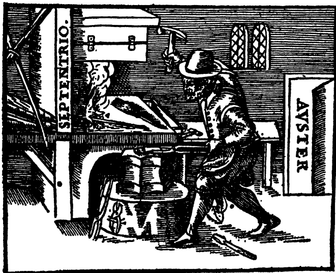
FIG. 12. GILBERT'S FIGURE OF A SMITH AT HIS ANVIL This illustrates Gilbert's discovery that a piece of red-hot iron placed on the north-south position ( septentrio-auster ) and struck by a hammer becomes magnetic. From the De Magnete .
